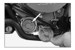
Insert a new oil filter in the engine case, grease the O-ring and mount the oil filter cover together with the O-ring. Tighten the screws to 6 Nm.
